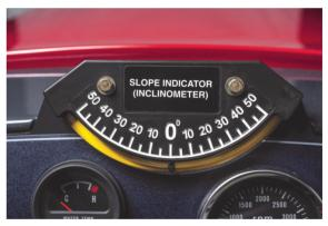
Integral tilt meter fitted as standard
