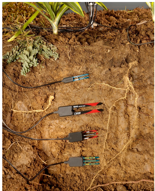
Picture 19: Volumetric water content sensors
