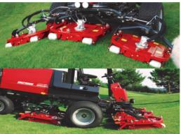
Each cutting deck can move freely, pivoting
