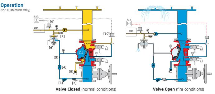
The BERMAD model 400Y-DP is held closed by water pressure in the control chamber [1]. Upon release of pressure from the control chamber, the valve opens.
