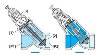
The Upstream Pressure [P1] applies balanced opening and closing hydraulic forces under the Diaphragm [1] and above the Plug [2]. Downstream Pressure [P2] applies hydraulic closing force under the plug, which seeks to reach equilibrium with the Set Spring [3] force. Should [P2] rise above setting, the hydraulic closing forces rise above the mechanical force of the spring, pushing the plug to modulate closed, reducing [P2] back to setting, and eventually shutting drip-tight.
