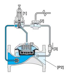
The Pressure Reducing Pilot [1] commands the Valve to throttle closed should Downstream Pressure [P2] rise above setting and modulate open when it drops below setting. The Hydraulic Relay Valve [2] closes upon receiving a remote pressure command, shutting off the main Valve.
