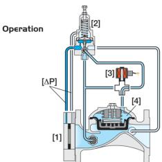
Pressure Differential [ $\Delta P$ ] across the Orifice Assembly [1] is in direct proportion to demand. The Flow Pilot [2] continuously senses [ $\Delta P$ ] and commands the Valve to throttle closed should demand rise above pilot setting. The Solenoid [3] hydrauliclly connects the flow pilot to the main Valve Control Chamber [4]. In response to an electric signal, the solenoid switches, directing line pressure into the control chamber causing the main Valve to shut.
