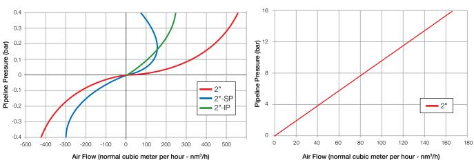
Air relief and intake charts refer to Side outlet and are based on actual measurements, made during 2014-2015 in Bermad Air Flow test bench, according to EN-1074/4 standard and certified to AS-4598 (2008) standard. Use Bermad Air software (www.bermad-air.com) for optimized Sizing & Positioning of Air Valves.
