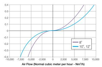
Air relief and intake charts are based on actual measurements, made during 2014 in Bermad Air Flow test bench, according to EN-1074/4 standard and refer to Down outlet. For Mushroom and Side outlet air flow performance, please consult with BERMAD.
