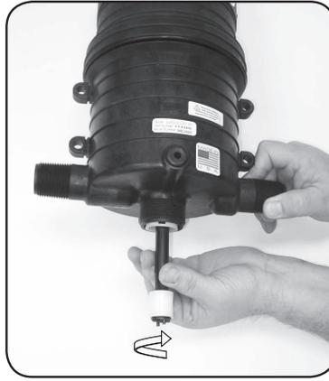
Step 2. Rotate #51 SHAFT 90° and pull from body.
